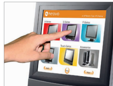
Scratch resistant touch panel with 5-wire Resistive touch technology
